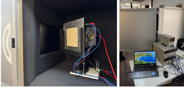
Fig. 7. X-band PDT phased array antenna demonstrator under test in Anyfields' EMBox XL.
