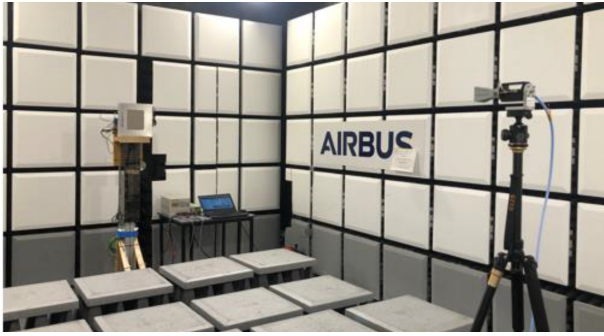
Fig. 3. X-band PDT phased array antenna demonstrator under test in a far-field anechoic chamber setup.
